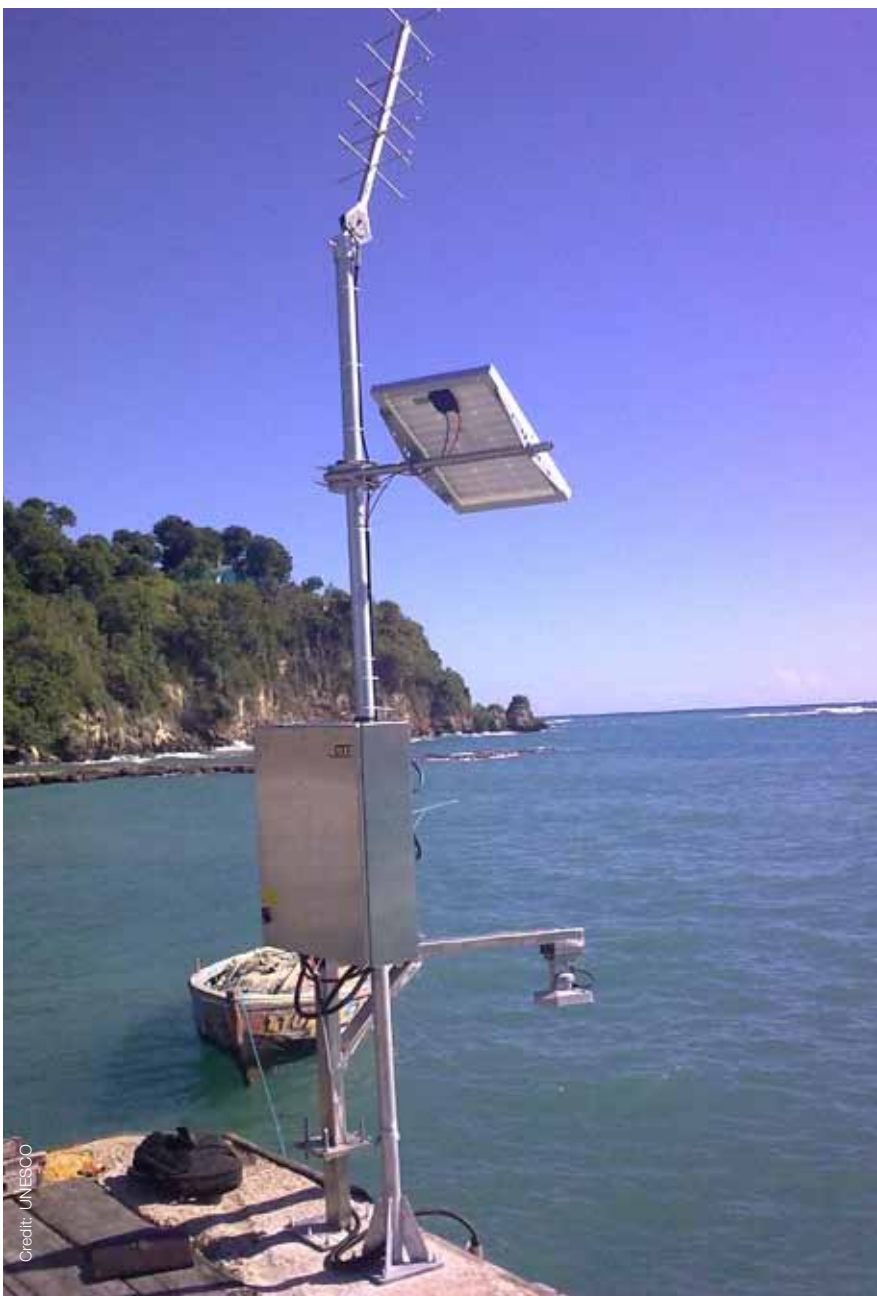
Sea Level Station installed by IOC in December 2013 in Jacmel, Haiti
