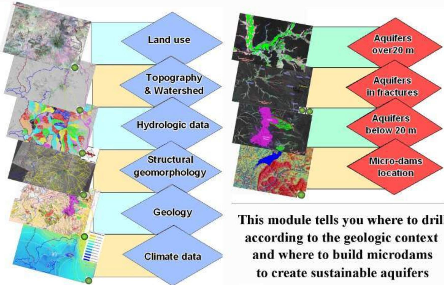
**This module tells you where to drill according to the geologic context and where to build microdams to create sustainable aquifers**
