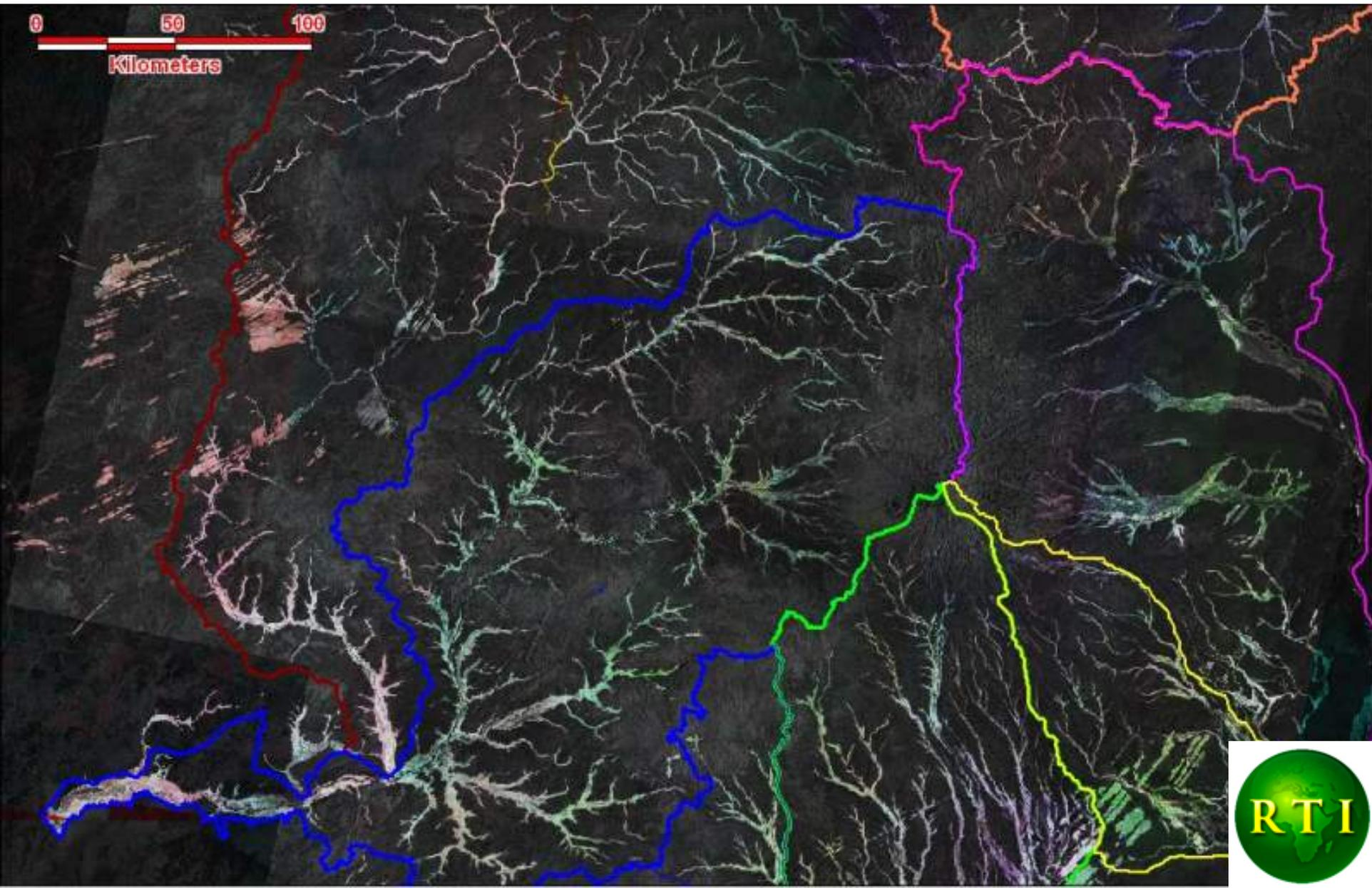
6- WATEX© eliminates false signals linked to clay deposits (green) using slope maps combined with Radar backscattering
