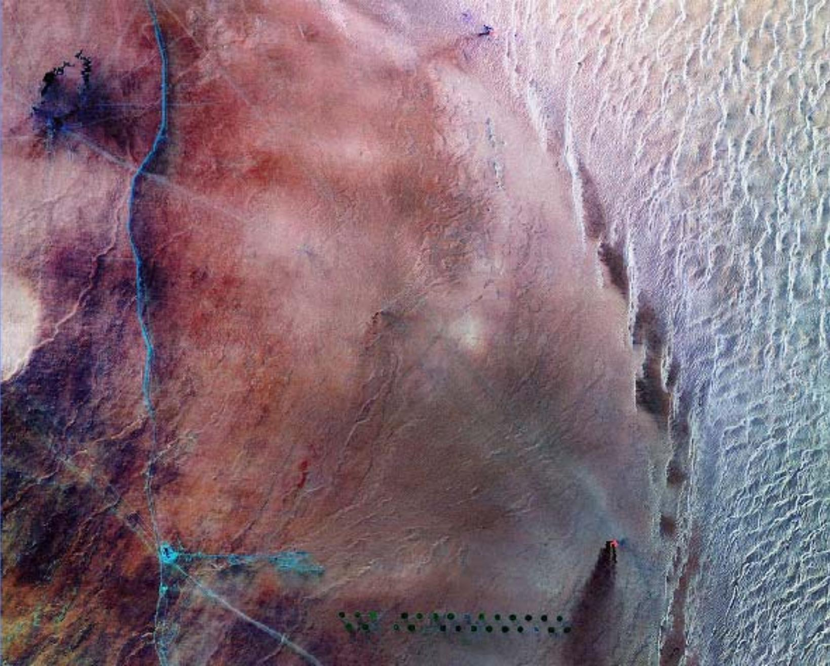
Water Leaks from the buried pipe were detected only by radar
