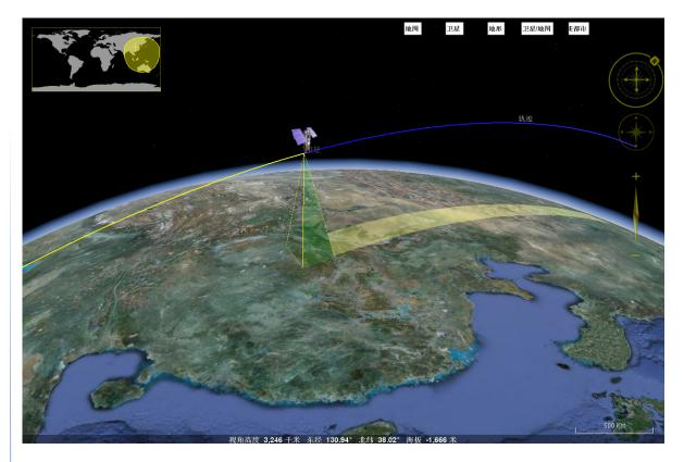
➤Compute the ephemeris data of various satellites, such as SPOT, Landsat, EOS AQUA/TERRA,FY and CBERS etc, from which the satellite's position and altitude, acquisition times, and its field of view can be obtained.
