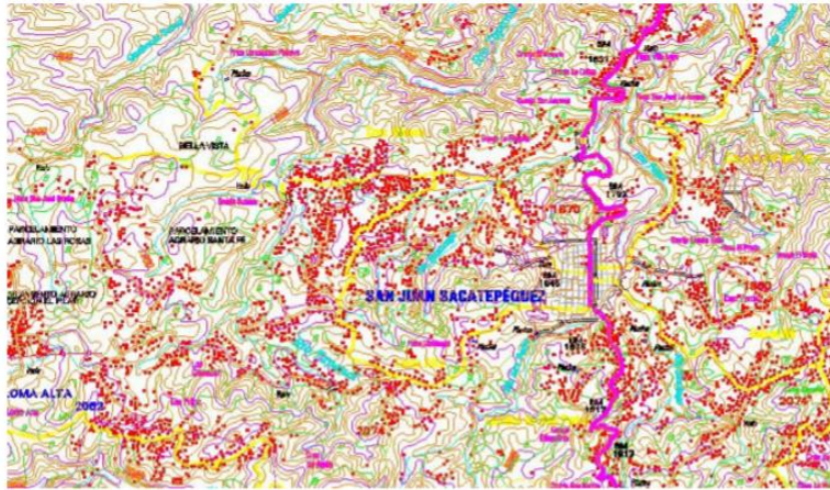
Figure 4.1-9 Compilation of 1:50,000 scale topographic map using MicroStation
