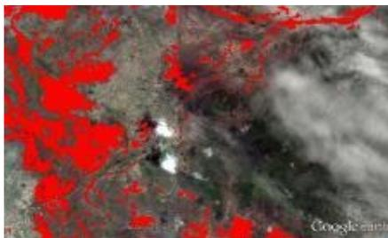
Radar-based flood mapping, which can make use of SAR satellite imagery, is a practice that can be applied globally. The recommended practice shows the use of SNAP software for pre-processing and processing of SAR imagery using a threshold method to derive the flood extent.
