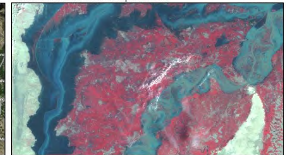
Flood Depth identified using PC (PC2, PC1, PC3 as RGB)
