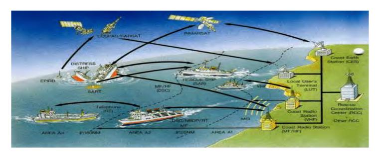
The GMDSS is an international system which uses terrestrial and satellite technology and ship-board radio-systems to ensure rapid, automated, alerting of shore based communication and rescue authorities and to ships in the immediate vicinity, in the event of a marine distress.
