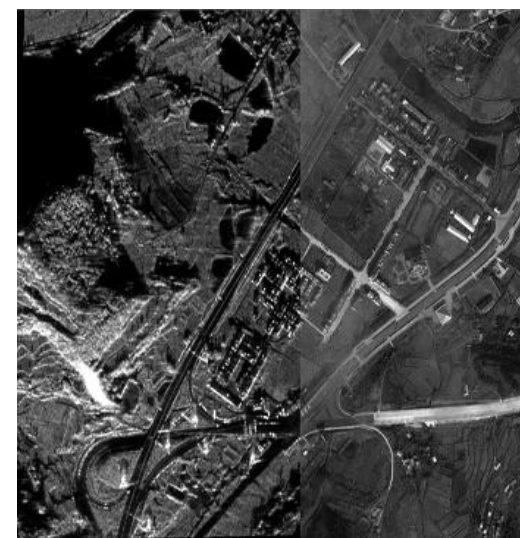
Registration result using liner features and Voronoi diagram
